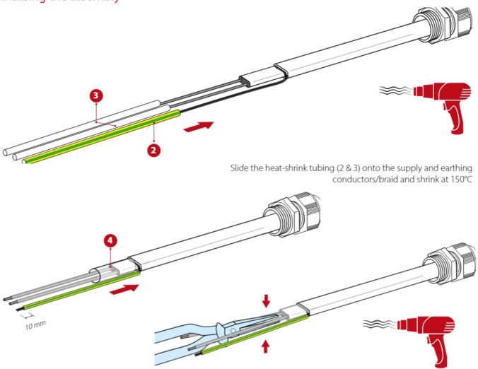
Slide on the heat-shrink tubing (4), shrink at 150°C and press together between the supply conductors with needle-nose pliers when warm
