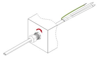
2. Screw the lower part of the cable gland into the junction box
