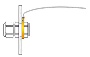
When installing metal cable glands in plastic enclosures: Earth the cable gland with an earthing kit!
