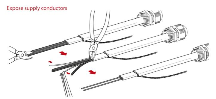
Carefully expose supply conductors &, if necessary, thoroughly clean
