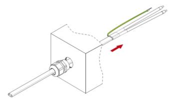
1. Insert the pre-assembled heating cable into the into the junction box
