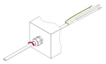
3. Position the seal and tighten the cable gland
