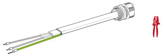
Push the wire end ferrules onto the supply conductors, push the pin terminal lug onto the braid and crimp using a suitable tool
